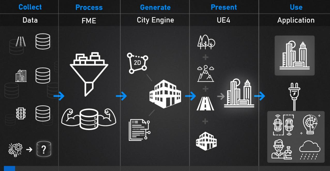
Fully automated process from geo data to a digital twin
